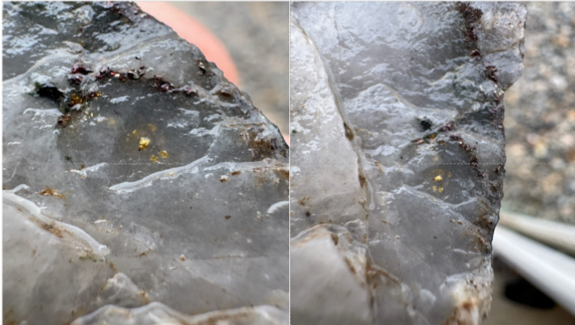
Visible gold identified in at-surface mineralised waste material at GDM's Challenger Mine, Adelong, NSW
